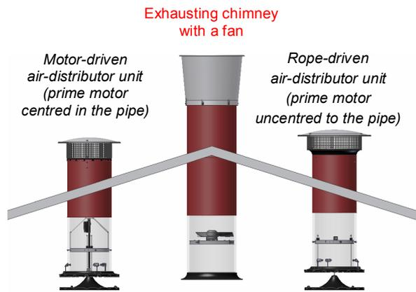
The air-distributor (AD) provides a steady fresh-air distribution in the livestock building. It is assembled just below the building roof and leads the fresh air from the outside through the roof area to the inside of the building. Here, the fresh air is subsequently delivered through the distributing disc and –ring.
