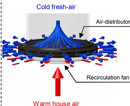
In extremely cold climate zones it can be advisable to use a recirculation fan. The latter can be ordered directly with the AD or be retrofitted any time.
