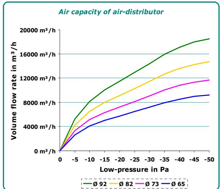
Fig. 1b: Diagram: air capacity of the AD at maximum opening level
