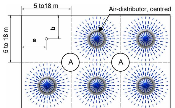
Fig. 2: Calculation and positioning of the AD
