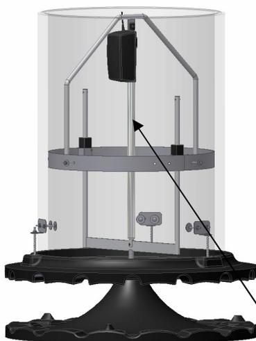
**Fig. E: air-distributor, wire drive**
