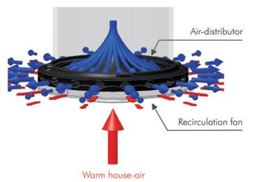
In particularly extreme climate zones, or with highly sensitive animal populations, it may be advantageous to additionally equip the air-distributor with a recirculation fan. This enables a more effective mixing of the cold fresh air with the warm house air, which is especially endeavoured in extremely cold winters.
